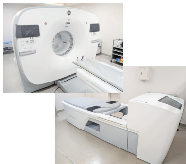
全身用PET-CT装置（左上）と頭部専用PET装置（右下） Whole-body PET/CT scanner (upper left) and dedicated brain PET scanner (lower right).
